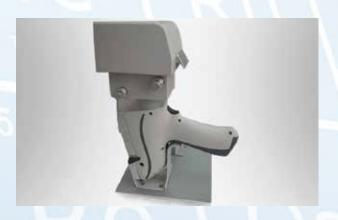
Use a laboratory stand to prevent X-Ray scattering when analyzing small objects or light matrix samples.
