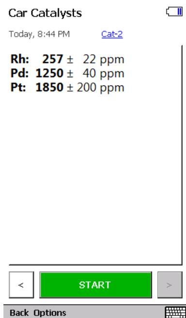
Figure 1. Measurement screen in Car catalyst testing mode.
