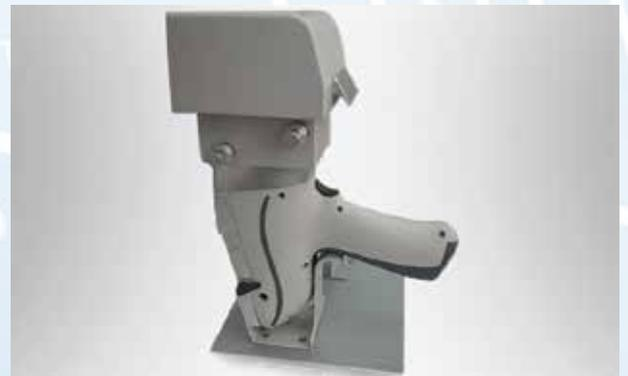
Use a laboratory stand to prevent X-Ray scattering when analyzing small objects or light matrix samples.
